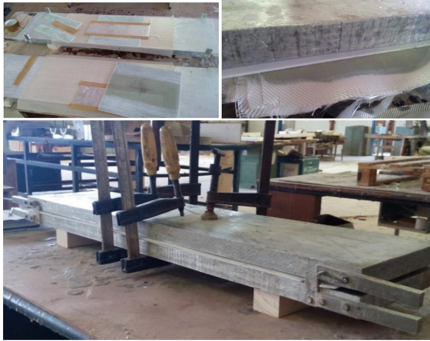
Figure 3-3 Forming of the composite plate in the tool
