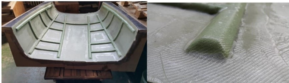
Figure 7-6 Sandwich construction of the lower engine cover in the female tool
