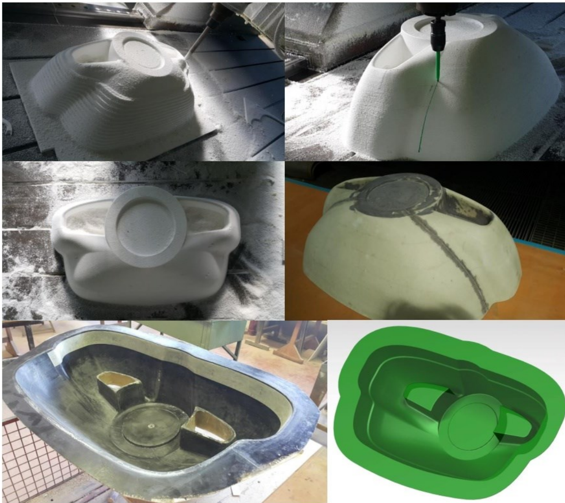
Figure 7-2 Front mask manufacturing on PHY machine, lamination and creation of conceptual design, female tool
