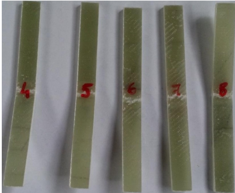
Figure 3-14 Fracture of bending test specimens
