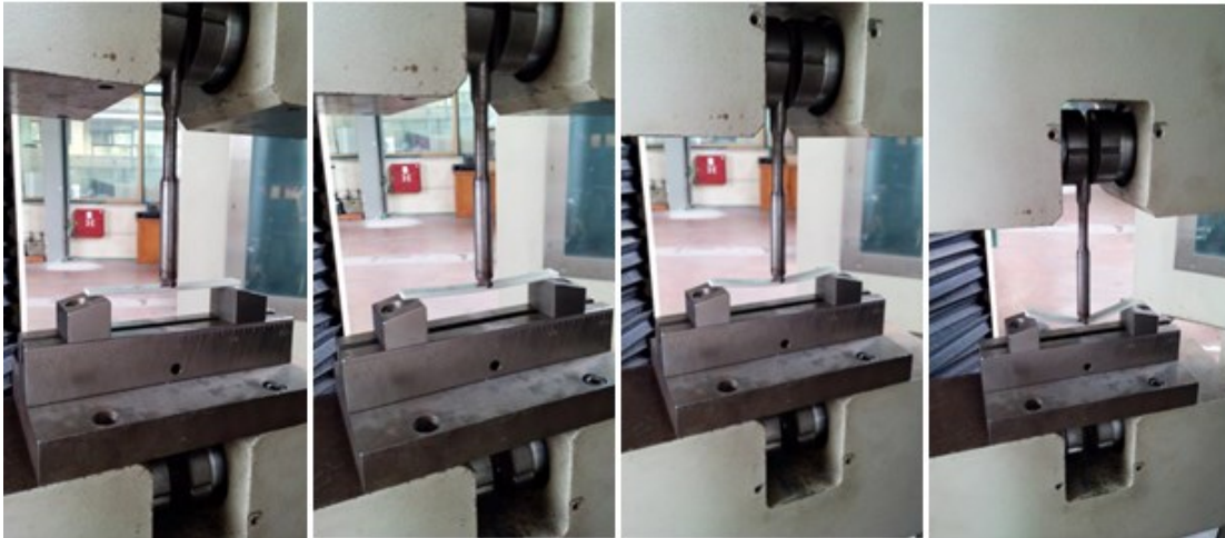
Figure 3-10 Electro-mechanical testing machine SCHENK TREBEL RM 200 (Bending test)
