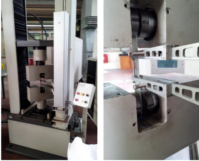
Figure 3-7 Electro-mechanical testing machine SCHENK TREBEL RM 200 (tensile test)
