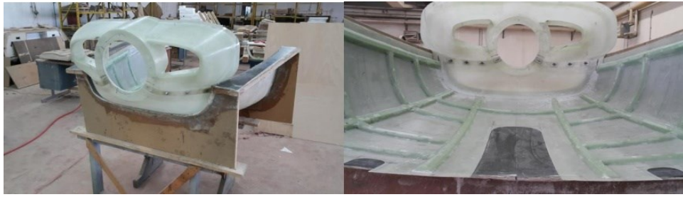
Figure 7-8“Gluing” of the lower engine coverwith the front mask
