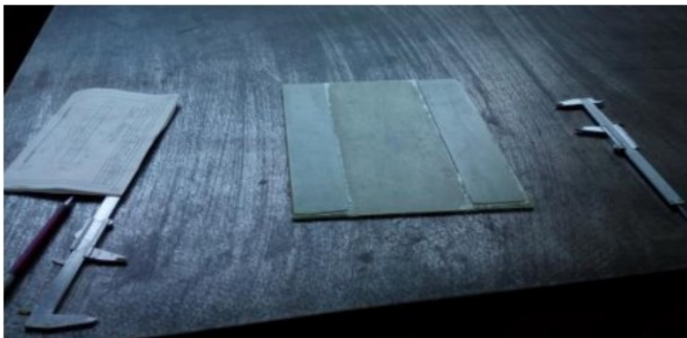
Figure 3-4 The laminate plate used for making the tensile test specimens
