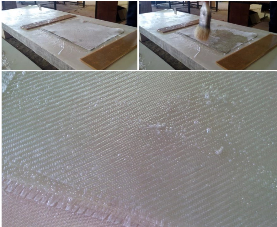
Figure 3-2 Assembling of fiberglass in tool
