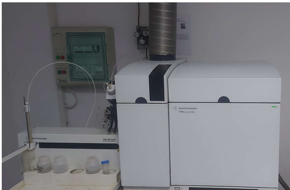
Slika 33. ICP-MS aparat Agilent 7700 ICP-MS (Agilent Company, USA)
