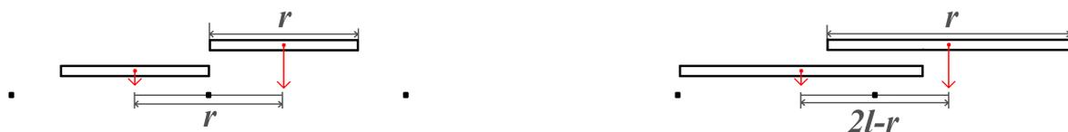
Figure 3.6: Illustration of equivalency of two models: (I) deposition of segments on localized adsorbing sites and (II) deposition of particles on extended lattice sites. On the left is a case of  $r < l$  and on the right a case of  $l < r < 2l$ .
