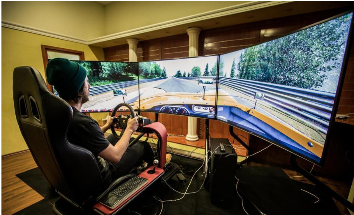
Figure 5.7. Nervtech 4DOF motion car driving simulator during a driving simulation. The image was taken and modified from [3]. (License: CC BY 4.0)
