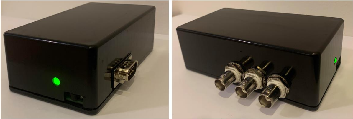
Figure 2.11. The prototype of improved EGG device in the plastic housing.
