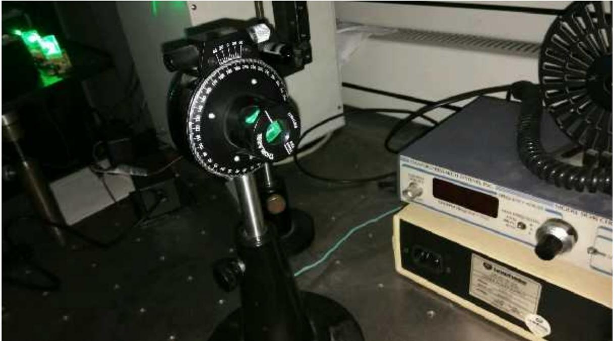
Figure 37 Polarizing prism.
