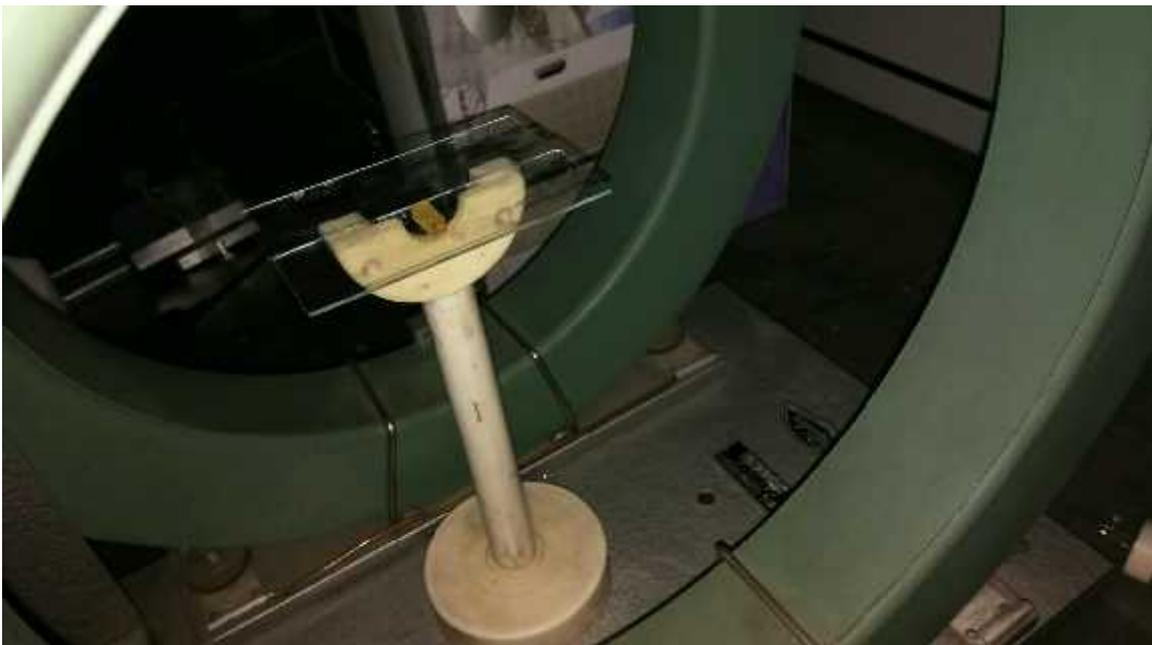
Figure 36 The mounting setup used to suspend the crystal in the Helmholtz coils magnetic field.
