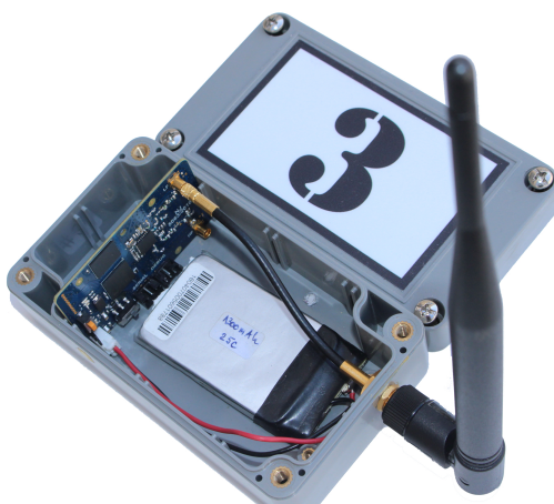
Figure 5.6: OdT mounted inside IP-67 rated enclosure.
