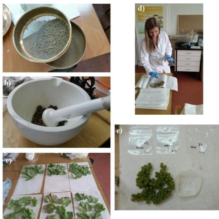
Figure 3.7 Soil sample preparation for the analyses: a) sieving through a 2 mm stainless sieve; b) grounding to a fine powder in an agate mortar with a pestle; c) the leaf drying d) the leaf grounding; and e) the grapevine samples preparation (separating the skin, pulp, seed and whole berries) for the elements' determination.
