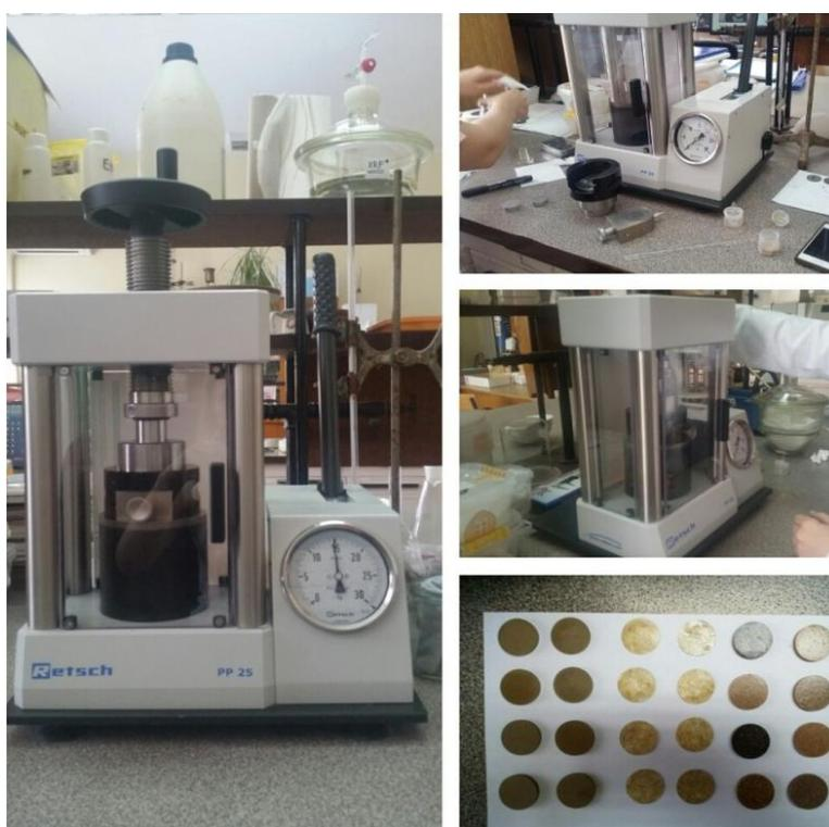
Figure 3.9 Soil and leaf preparation of the pellets for the element analysis by WD-XRF.
