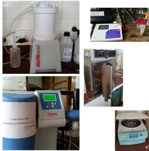
Figure 8.1.1 a) distillator for preparing acid (p.a.) for the samples digestion; b) distillator for preparing ultra-pure water used for the samples preparation; c) pH-meter d) dryer; e) centrifuge.
