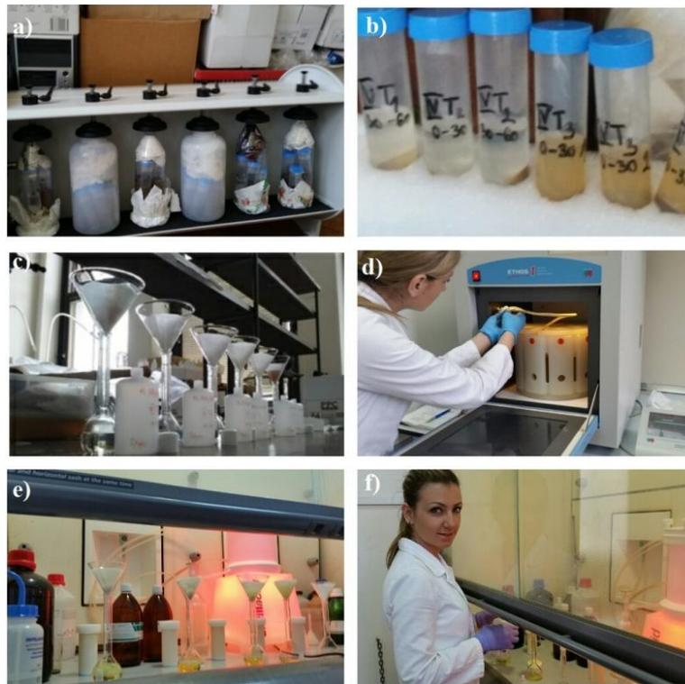
Figure 3.8 a) Soil extraction on the rotary shaker; b) centrifuged (left three cuvettes) versus non-centrifuged (right three cuvettes) soil extracts; c) the supernatants separating from the precipitate through the filter paper after the extraction; d) soil and plant material microwave digestion; e) filtering and packing in polyethylene bottles after the soil and the plant material microwave digestion.
