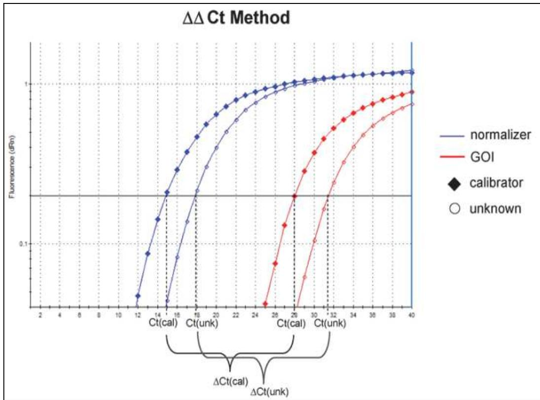
**Figure 19:** The Calculation of  $\Delta Ct$  using  $\Delta\Delta Ct$  method, where  $\Delta Ct$  is determined by calculating the difference between the Ct of the normalizer and Ct of the GOI for each sample (source: Agilent Technologies “Introduction to Quantitative PCR: Methods and Applications Guide” (2016)).
