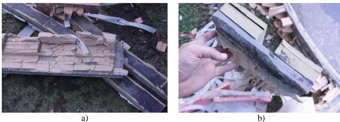
Figure 5.84 a) Strong glued connection between the U-shaped elastomers and bricks and b) between two layers of elastomer
