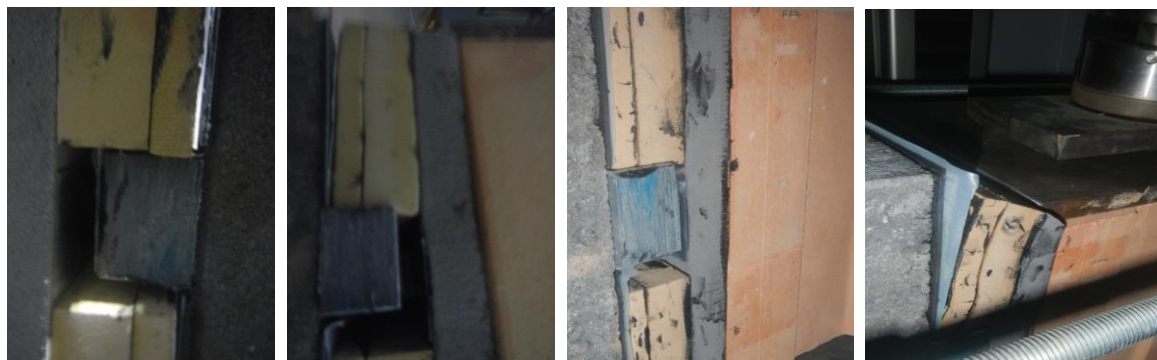
Figure 4.26 Deformations at different load levels of the Test C
