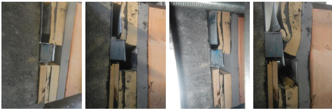
d = 5.9 mm (1 kN) d = 12.4 mm (2 kN) d = 22.3 mm (3.5 kN) d = 29.0 mm (4.9 kN)
