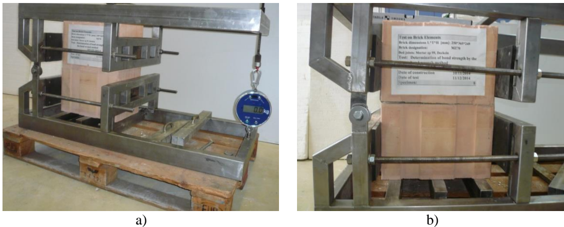
Figure 4.7 a) Determination of bond strength of the mortar-unit interfaces and b) bond failure at the end of the test
