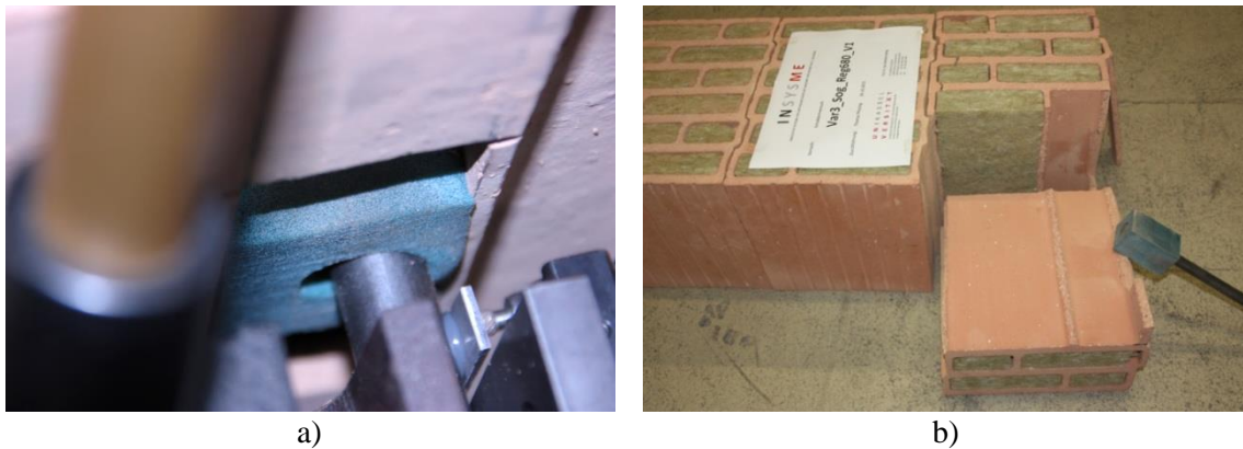
Figure 4.17 a) Deformation of the elastomer during the test and b) splitting of the brick in a case of connection type 3 (INSYSME, 2017a)
