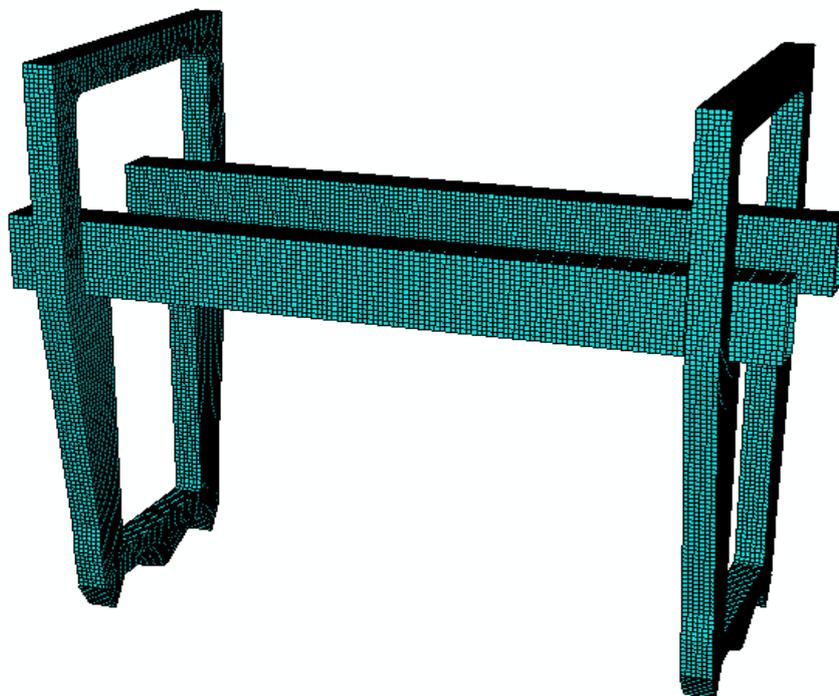
**Figure 1.2** A FE model of the transporter crane
