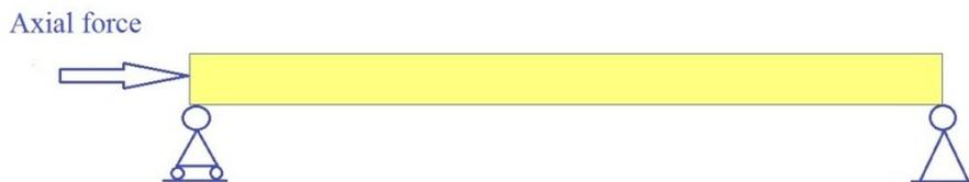
**Figure 5.5** Loading configurations of a simply supported hollow beam-column
