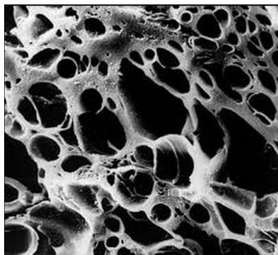
**Figure 2.8.** SEM images of an activated carbon materials [43].
