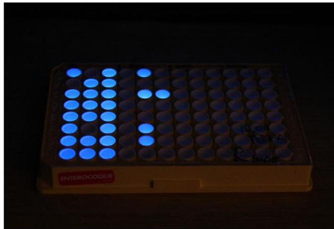
**Fig 3.7** BIORB MPN system for detection of enterococci
