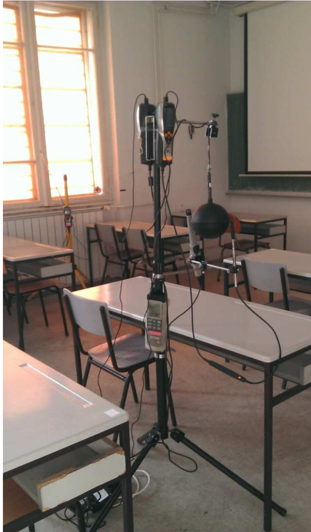
Figure 10. The easel position M05 with black globe, IAQ and HOT wire probe.
