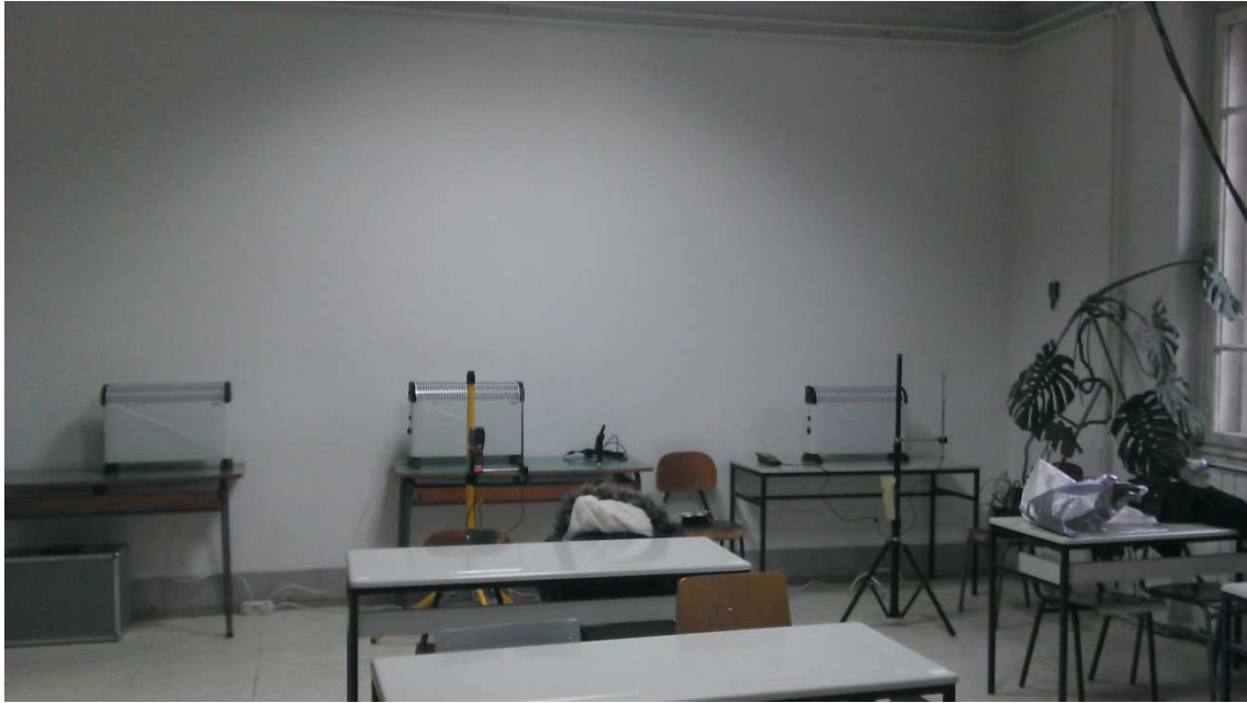
Figure 11. Additional electrical heaters with hot wire and turbulent probe instruments
