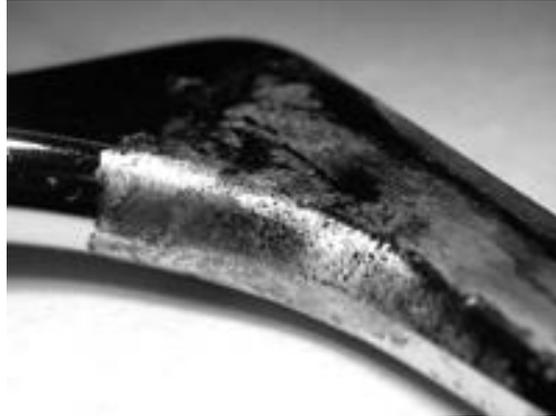
*Figure 3.5. Corrosion of a metal implant used for total hip replacement, [5]*
