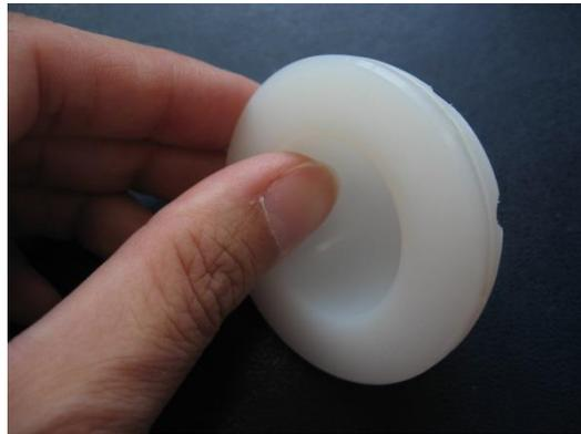
*Figure 2.8. Component of hip implant made of UHMWPE, [9]*
