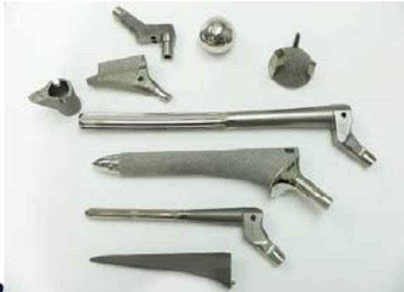
*Figure 2.6. Prosthesis made of Ti alloys [10]*
