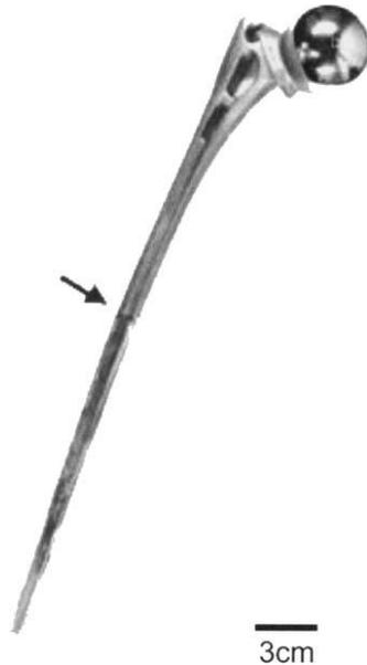
*Figure 3.7. An example of a broken prosthetic base of a hip prosthetic 9 years after implantation, [130]*
