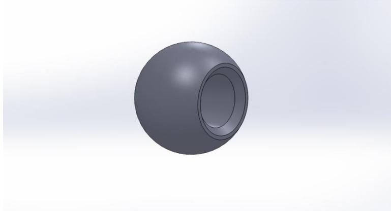
*Figure 7.9. Hip implant 3 cup - solid model*
