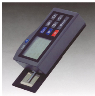
Slika 6.2.16.1. Portabl Surface Roughness Tester TR200
