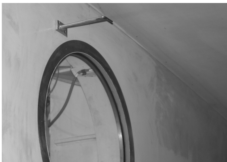
Sl. 50. Nova pito-sonda u radnom delu aerotunela T-38
